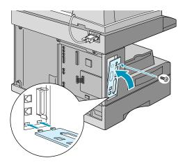
**9** Insert the network interface card, ensuring that the network cable connector and LEDs on the card align with the port and LED slots.
